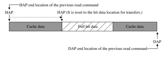
2) The read requested data is transferred, and a new read-ahead operation is not performed.
